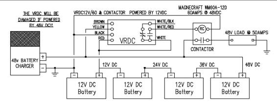
The VRDC 12V-60 senses when the battery bank is being discharged below a minimum threshold point and acts as a low voltage disconnect, disconneing the load to allow the battery charger to charge the batteries. It reconnects the loads when the batteries have been charged. The time delay prevents the loads from being disconnect early due to temporary battery voltage drop due to switching loads.
