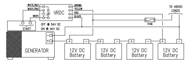
The VRDC 12V/60 senses when the battery bank is being discharged below a minimum threshold point and starts the generator to charge the batteries. It shuts off the generator when the desired battery voltage is achieved. The time delay prevents the generator from starting on temporary battery voltage drops due to switching loads.
