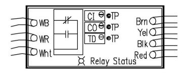
The test points shown are for field calibration of the cut in, cut out, and time delay potentiometers.
