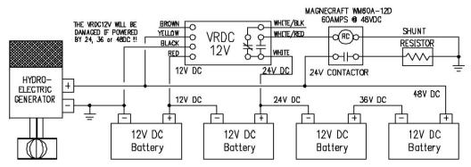
The VRDC 12V-60 senses the battery voltage and activates a contactor to shunt the excessive power thru a load shunt resistor to prevent an over voltage condition. The VRDC 12V-60 must be powered by 12VDC from the battery bank even though it is sensing the full battery bank voltage level.
